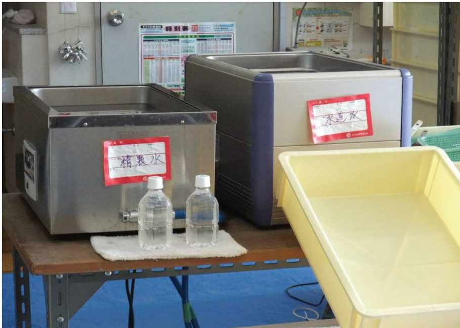
Fig. 9 The items first had to be rinsed gently in tap water (right), and then in purified water (left) (Copyright: The Rikuzentakada Municipal Museum)
